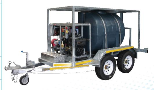
Heavy Duty - DIESEL - Hot Water - 3625 PSI, 15LPM
